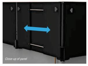
Panels are adjustable to fit almost any optical table
